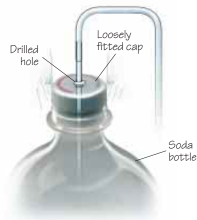
LOOSELY FITTED CAP on the soda bottle (above) allows the escape of air injected through the central tube but does not let contaminants fall in. A rubber stopper with a bent tube set in one of its two holes (right) provides the same function on the watercooler jug.
